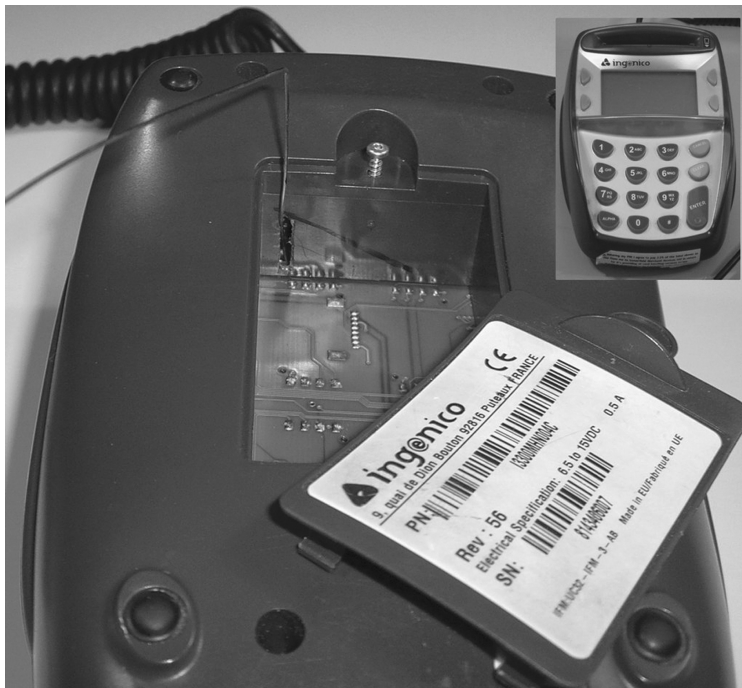
Figure 10.4: A rigid wire is inserted through a hole in the Ingenico’s concealed compartment wall to intercept the smartcard data. The front of the device is shown on the top right.
